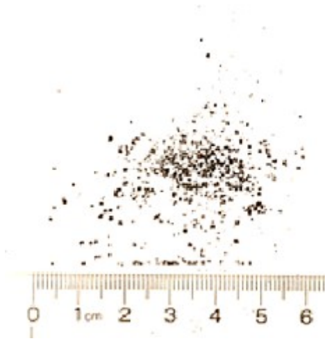
Figure 3. Gun Power Grains from the FHS Cartridge.
